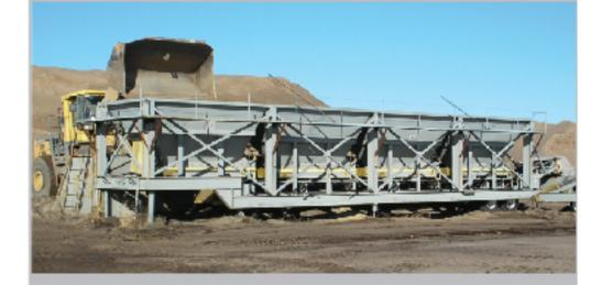
Our four-bin Accublender™ is used to create these mixes. It features a computerized blender with an on-board screen deck that removes oversized particles and a mechanical paddle wheel that ensures uniformity. It automatically adjusts for flow rates of material and stops the conveyor belt when feed bins need to be replenished.
