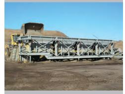
Our four-bin Accublender™ is used to create these mixes. It features a computerized blender with an on-board screen deck that removes oversized particles and a mechanical paddle wheel that ensures uniformity. It automatically adjusts for flow rates of material and stops the conveyor belt when feed bins need to be replenished.
