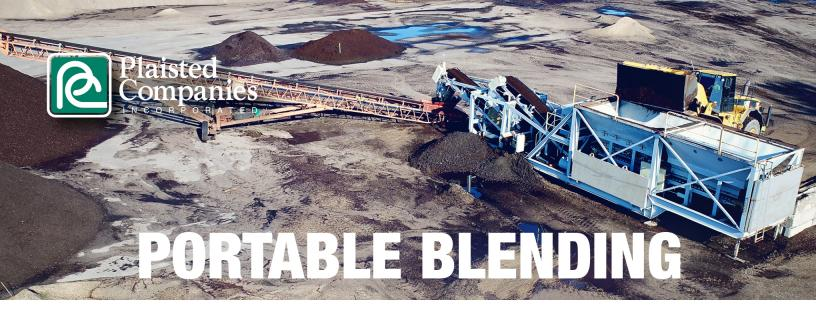
As *Soil Experts*, Plaisted Companies can provide portable blending solutions between construction and landscaping development. The *Accublender*  $^{TM}$  2 is a portable two-bin blender capable of blending up to 2,500 tons of material a day on-site. This is ideal for locations where acceptable materials are available to blend and there is sufficient space.
