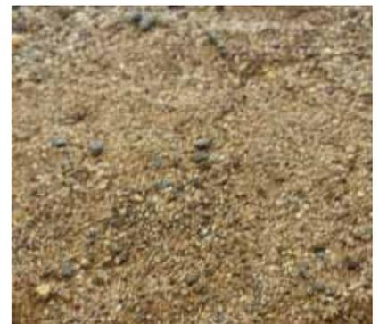
*The iron aggregate used in our iron-enhanced sand blend is produced by Connelly-GMS, Inc. This product, designed to meet standards developed using EnviroMetal Technologies, Inc. (ETI) patented technology, has been proven effective in laboratory testing and in over 100 full-scale systems.*
