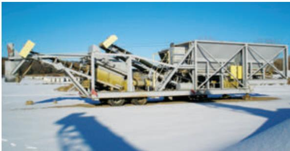
The Accublander™ 2 is a portable two-bin blender capable of blending up to 2,500 tons of material a day on your site. This is ideal for locations where acceptable materials are available to blend and there is sufficient space.
