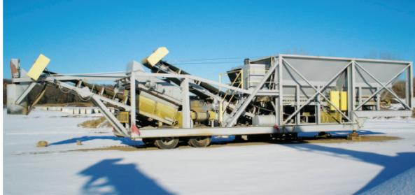
Accublender 2 two-bin blender can produce up to 2,500 tons of material a day on your site.
