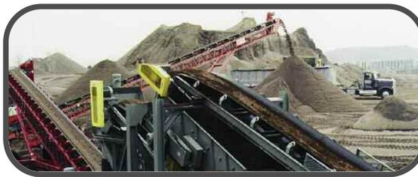
The **Accublender™** is a unique computerized blender that has an on-board screen deck that removes oversized particles and a mechanical paddle wheel that insures uniformity. The **Accublender™** automatically adjusts for flow rates of material and will stop the conveyor belt when feed bins run out of material.
