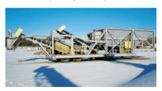
The Accublender<sup>™</sup> 2 is a portable two-bin blender capable of blending up to 2,500 tons of material a day on your site. This is ideal for locations where acceptable materials are available to blend and there is sufficient space.
